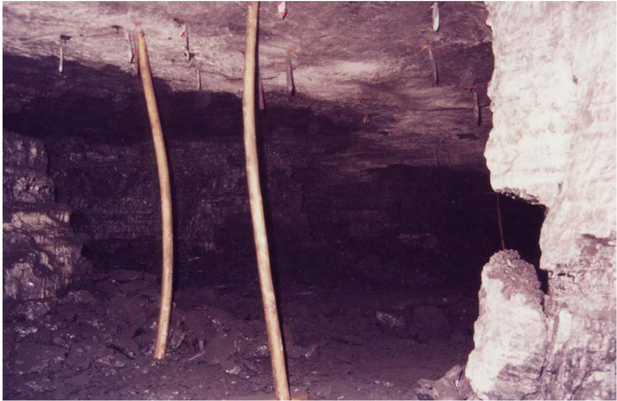
Figure 13 - Timber props acting as only convergence indicators, (Madden, 1989)
