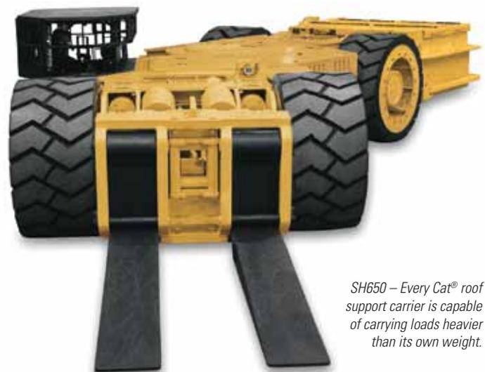
*SH650 – Every Cat® roof support carrier is capable of carrying loads heavier than its own weight.*
