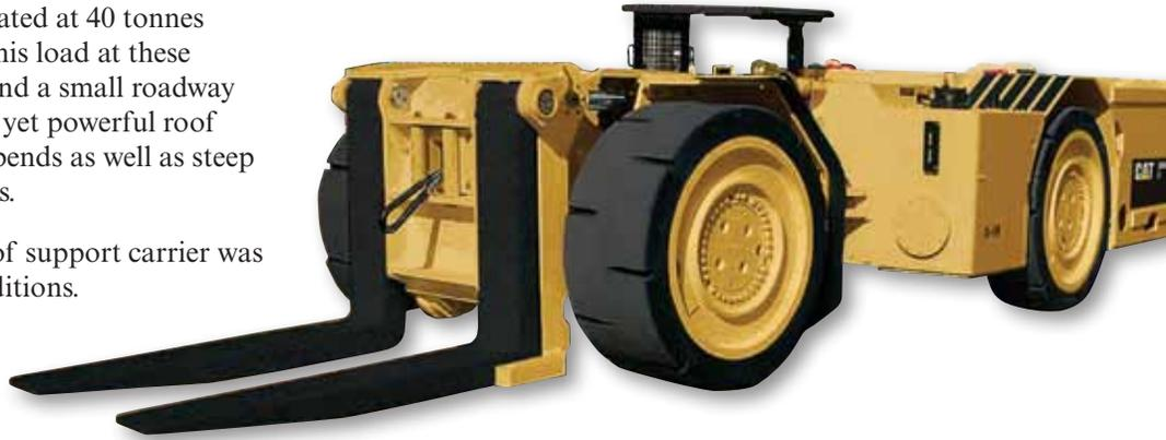
*The SH640 D comes ready to operate with heavy-duty forks as standard. A range of attachments is available to turn the SH640 D into a utility vehicle between longwall moves.*
