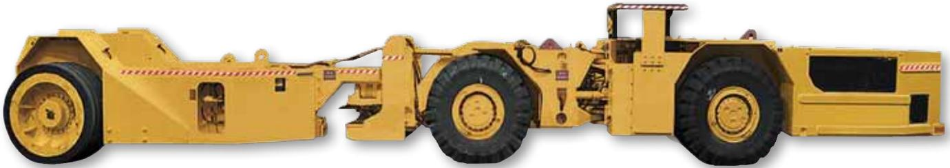
SH150 roof support trailer for CL10 and CL15 models
