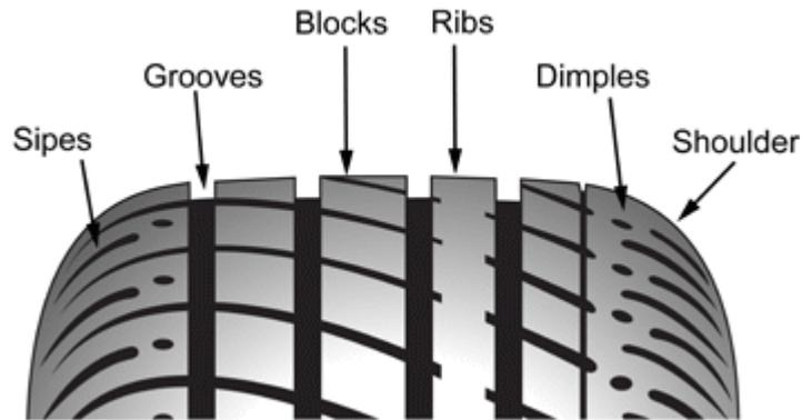
**Sipes** are the small, slit-like grooves in the tread blocks that allow the blocks to flex. This added flexibility increases traction by creating an additional biting edge. Sipes are especially helpful on ice, light snow and loose dirt.
