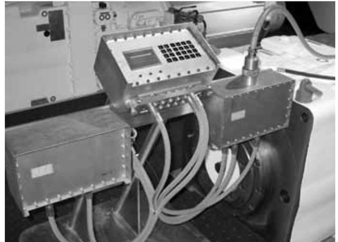
*Configuration of PMC™-D and PMC™-V connected to a CST drive*
