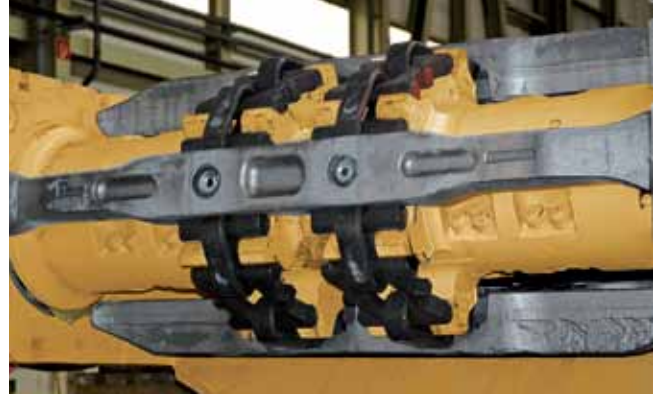
PowerChain and sprocket in use with a Cat beam stageloaader
