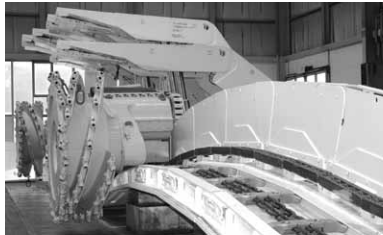
Simulation of a hump during a compatibility test with a shearer
